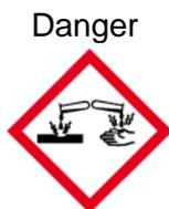
**Hazard statements:** Skin Corr. 1: H314 - Causes severe skin burns and eye damage. Met. Corr. 1: H290 - May be corrosive to metals.
